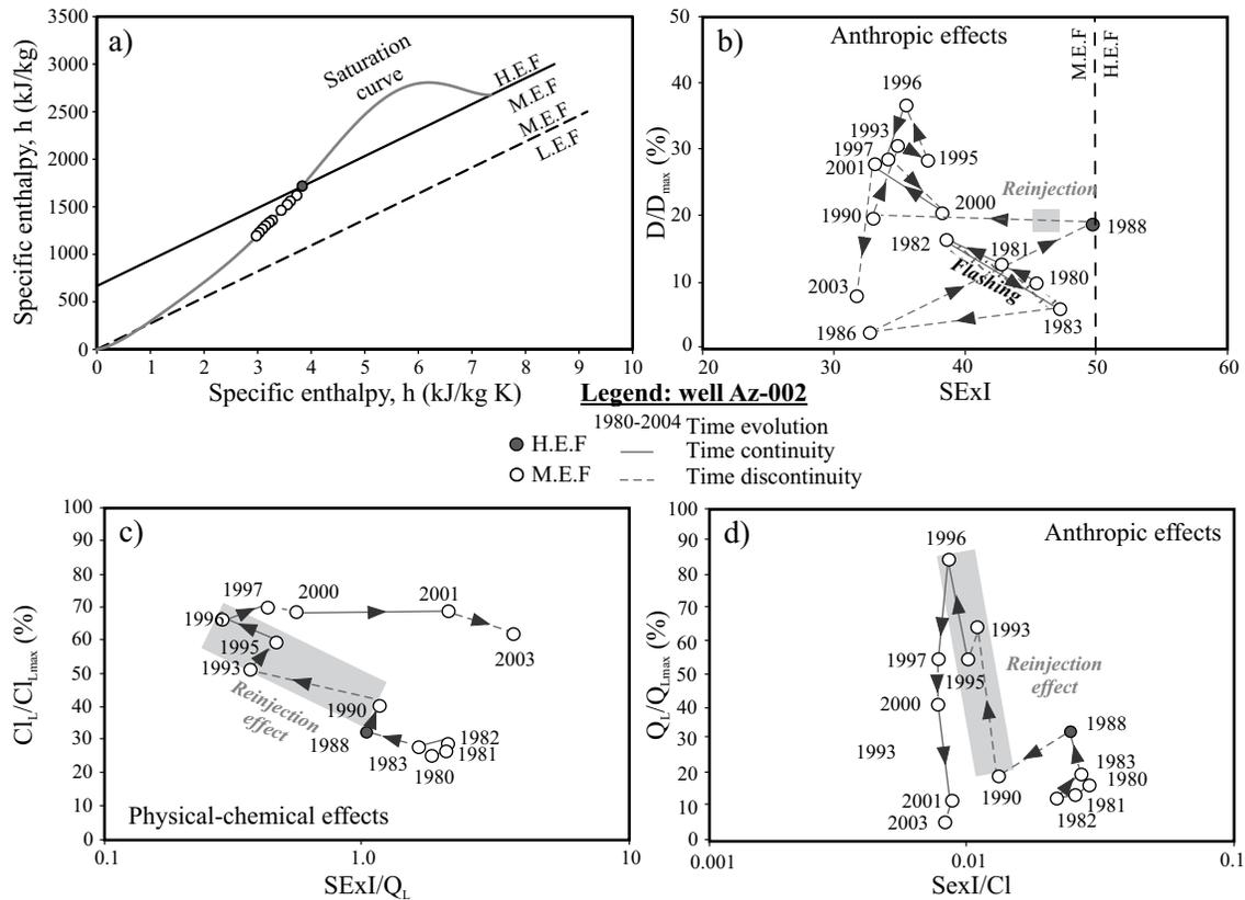
Figure 6. Az-002 well plots. a) Lee's SExI plot; b) OE plot:  $D/D_{max}$  vs. SExI; c) CE plot:  $Cl_L/Cl_{Lmax}$  vs.  $SExI/Q_L$ ; d) the normalized  $Q_L$  ( $Q_L/Q_{Lmax}$ ) versus SExI/Cl plot ( $Q_L$  effect, QE). The thick solid and the dotted lines indicate the position of the low (L.E.F.), medium (M.E.F.) and high (H.E.F.) exergy fields, following the criteria of Lee (1996). See text for discussion.
