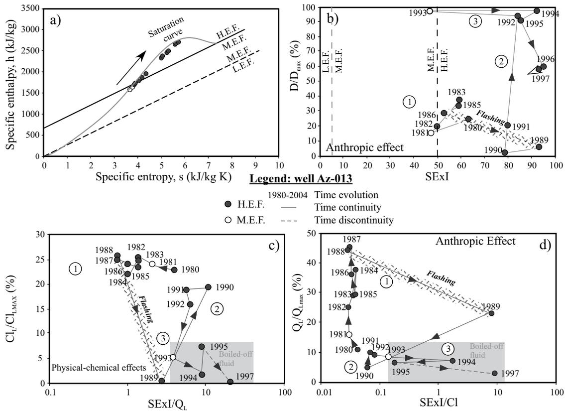
Figure 5. Az-013 well plots. a) Lee's SE<sub>X</sub>I plot; b) OE plot:  $D/D_{max}$  vs. SE<sub>X</sub>I; c) CE plot:  $Cl/Cl_{Lmax}$  vs. SE<sub>X</sub>I/ $Q_L$ ; d) the normalized  $Q_L$  ( $Q_L/Q_{Lmax}$ ) versus SE<sub>X</sub>I/ $Cl$  plot ( $Q_L$  effect, QE). The thick solid and the dotted lines indicate the position of the low (L.E.F.), medium (M.E.F.) and high (H.E.F.) exergy fields, following the criteria of Lee (2001). See text for discussion.
