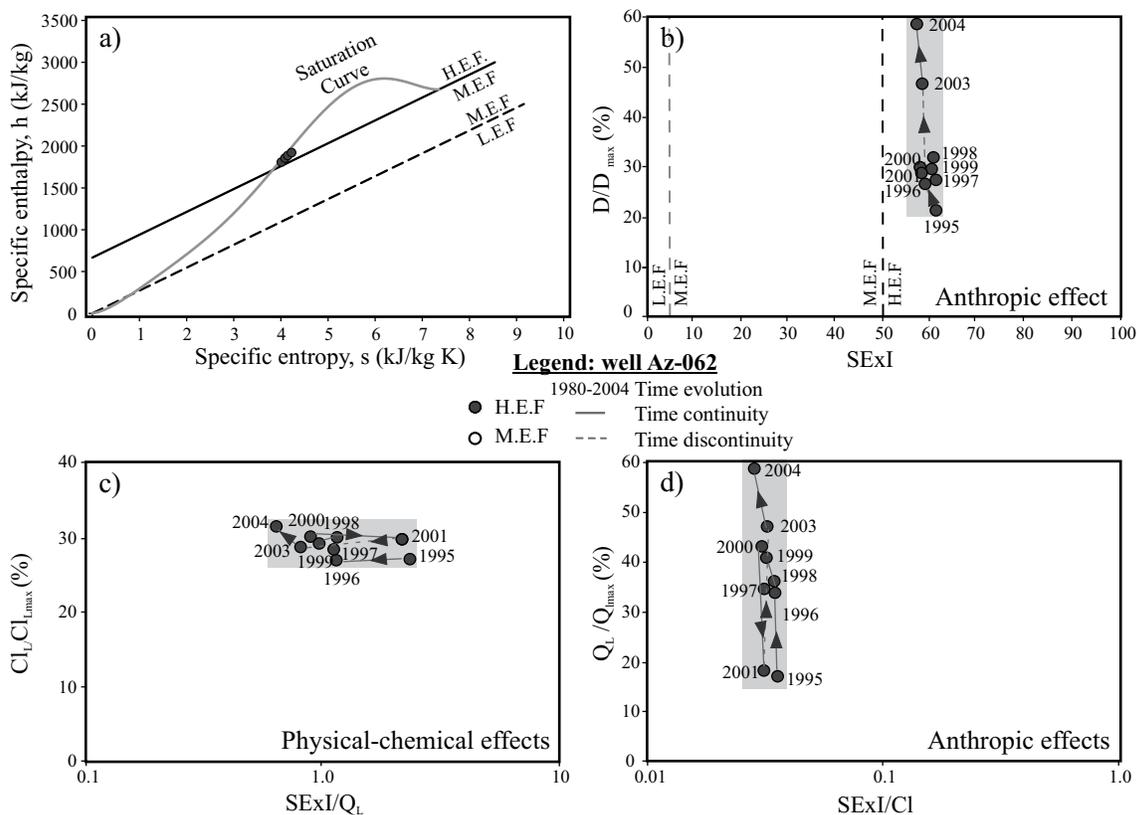
Figure 4. Az-062 well plots. a) Lee's SExI plot; b) OE plot:  $D/D_{max}$  vs. SExI; c) CE plot:  $Cl_L/Cl_{Lmax}$  vs.  $SExI/Q_L$ ; d) the normalized  $Q_L$  ( $Q_L/Q_{Lmax}$ ) versus SExI/Cl plot ( $Q_L$  effect, QE). The thick solid and the dotted lines indicate the position of the low (L.E.F.), medium (M.E.F.) and high (H.E.F.) exergy fields, following the criteria of Lee (2001). See text for discussion.
