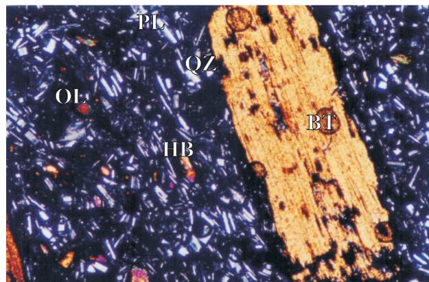
Figure 9. Microphotograph of a sample from the Cerro Gordo dacitic dome. OL: Olivine, PL: Plagioclase, QZ: Quartz, BT: Biotite, HB: Hornblende.
